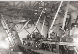
Coal washing machine using a flat belt (machine for the process of washing coal to remove impurities)
